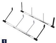
Slide the T and J joiners onto separate support poles, spacing the joiners evenly as shown.
