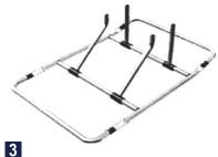
Insert the **U frames** onto the ends of both side frames.
