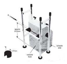
Mark the locations where you will fit the mounts on the front of your console (placing them as far apart as possible). Mark the console **side mounts** position (as high as possible)
